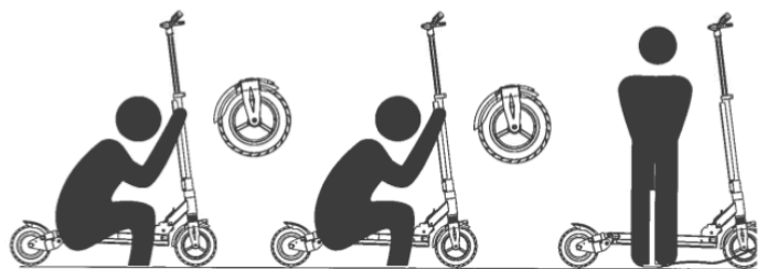
If the main rod shakes during the running, please tighten the nuts for clamp and secure it.
