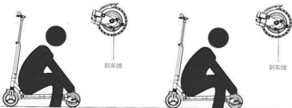
If the brake is too tight, please use M5 hex wrench to loose the screw of the disc brake holder by anticlockwise direction, and short the brake cable, then fix the screw tightly; if the brake is too loose, just loose the screw and make the brake cable to be longer and then fix the screw tightly.
